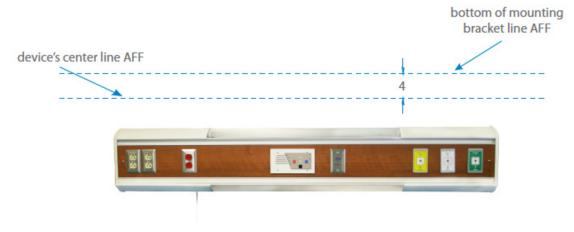
3. Using a stud locator, mark the location of any metal studs or blocking in the building wall that intersect the console mounting location.
