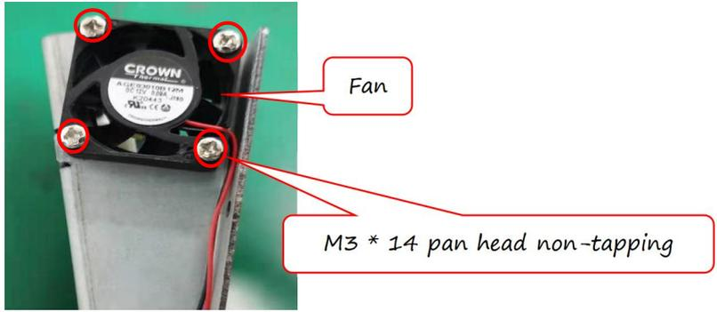
3. Plug the fan cable through the slot in the main holder into the J4 socket on the printing power board, connect the AC-DC connection cable to the power board and the printing power board, and plug the keypad cable into the J12 socket on the printing power board; snap the magnetic loop into the printer cable, and then plug the
