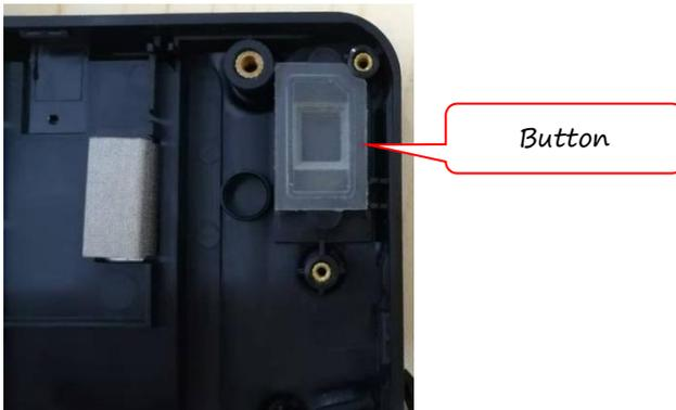
2. Position the light transmitting column on the front housing.
