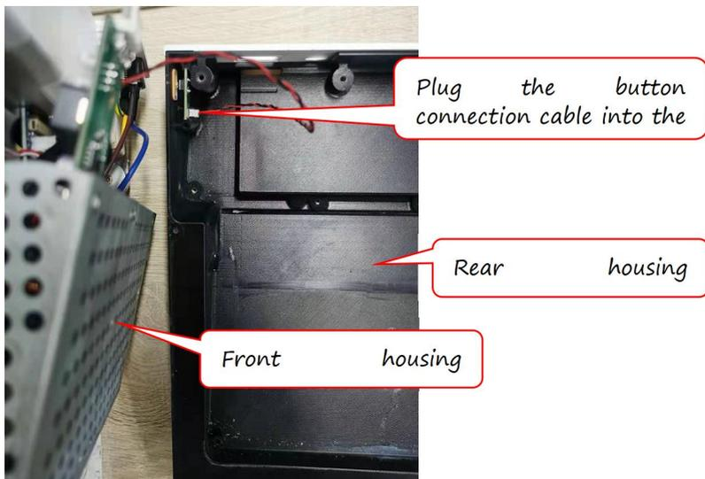
2. Install the front and rear housings together.
