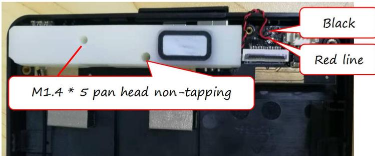
**Note:** The positive and negative electrodes of the loudspeaker line must be soldered correctly.
