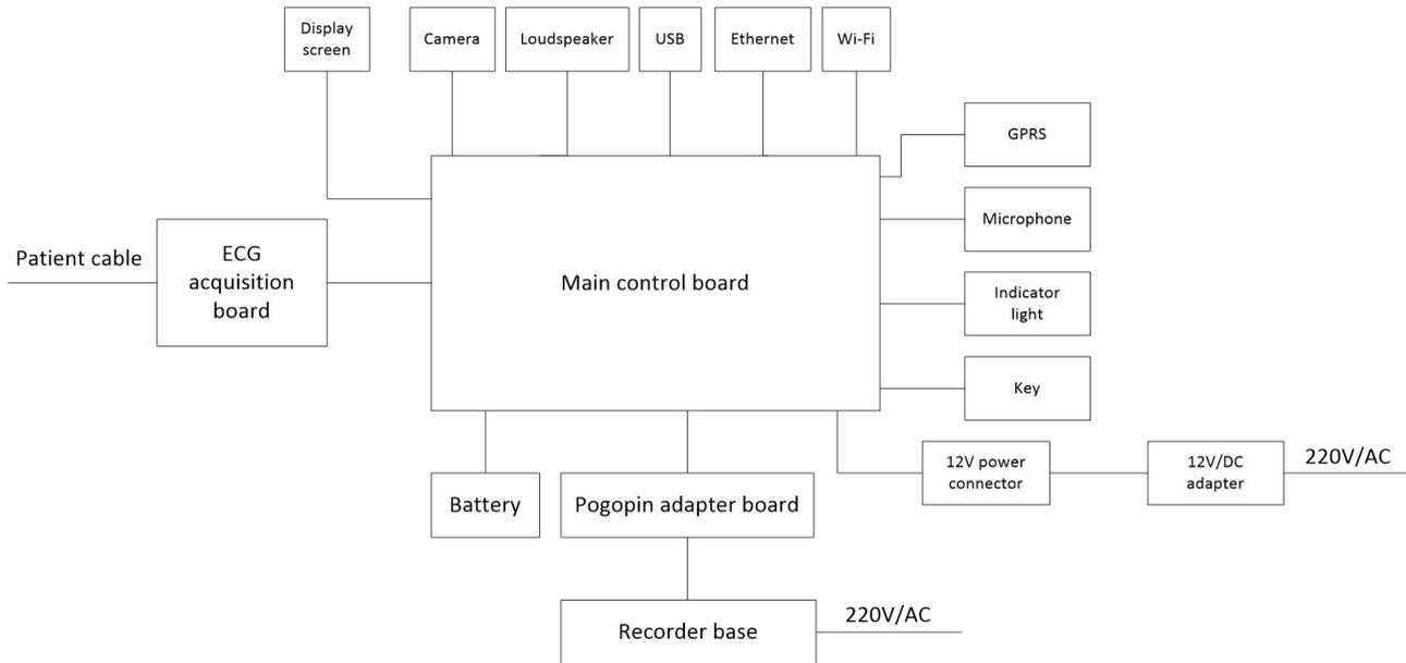
*Structure block diagram of 10.1" model device (with recorder base)*
