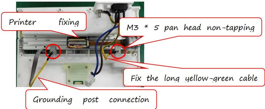
**Note:** Pay attention to the installation of the printer fixing spacer to ensure that the bent side is facing downwards; the fixing spacer should be pressed in place on the metal housing of the thermal print head.
