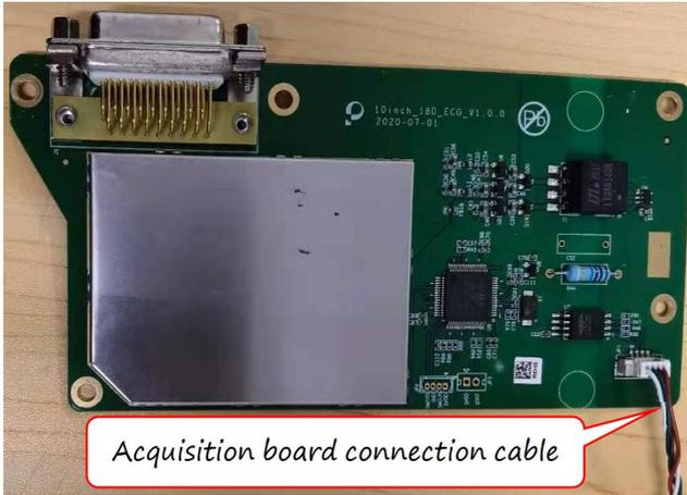
2. Snap the acquisition board into the corresponding position on the front housing and fix it with five M2 \* 5 pan head non-tapping screws without any adverse phenomena such as slipping or loosening.
