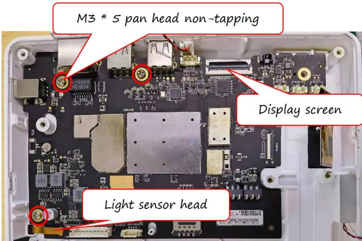
**Note:** The light sensor head FPC cannot be squashed under the main control board.
