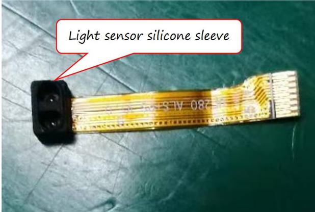
2. Attach the light sensor to the corresponding position on the front housing and glue it in place.
