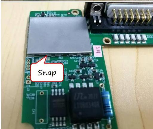
*Note: The edges of the shielding cover must snap into place.*
