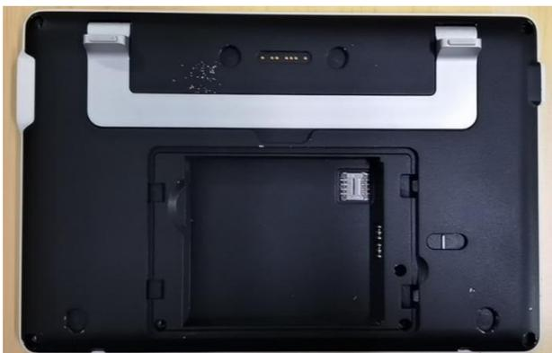
*Note:* There should be no gap around the closed housing, and the snaps should fit into place.
