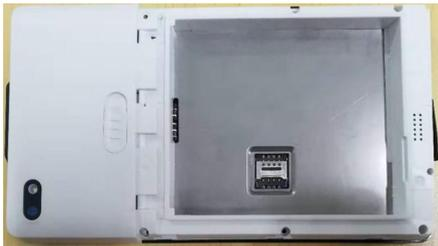
**Note:** There should be no gaps anywhere, and the snaps should be snapped properly into place.
