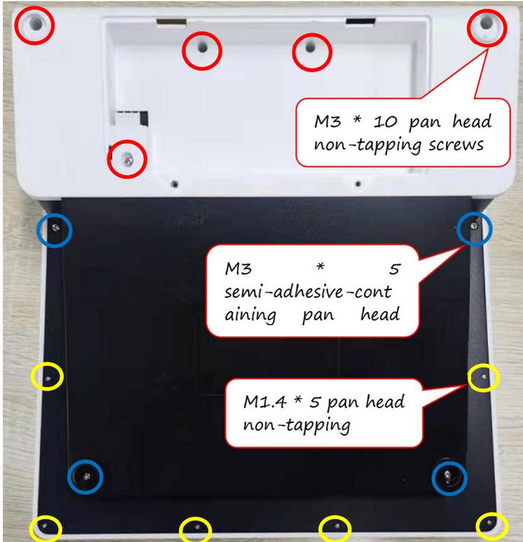
*Note: The M1.4 \* 5 pan head non-tapping screws shall be twisted manually with a screwdriver.*
