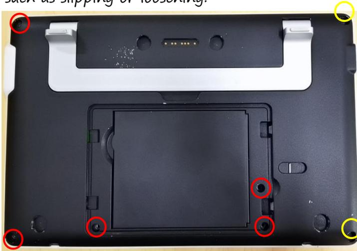
*Note: Those marked with red circles are M3 \* 5 pan head non-tapping screws, yellow circles are M2 \* 5 pan head non-tapping screws.*
