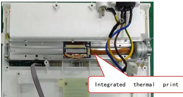
2. Flip the front housing over and secure the integrated thermal print head with three M3 \* 5 semi-adhesive containing pan head non-tapping screws.
