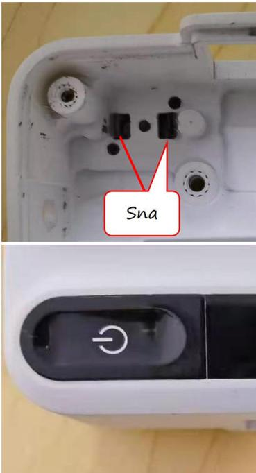
**Note:** The snap on the back of the button holder should be attached onto the front housing.
