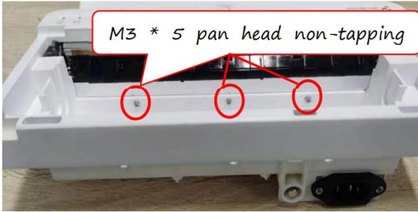
3. Flip the front housing back, install the paper compartment cover open button to the left side of the front housing, align the hole of the paper compartment cover open button with the metal post of the integrated thermal print head, then push in the paper compartment cover open button and manually twist one M1.4 \* 5 pan head non-tapping screw in place.
