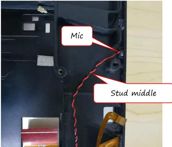
2. Install mic into the corresponding slot on the front housing.
