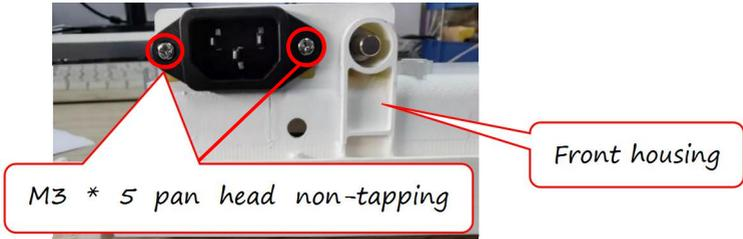
**Note:** Install the AC socket with triangular pins facing downwards.
