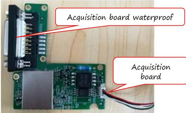
5. Snap the acquisition board into the corresponding position on the front housing and fix it with five M2 \* 5 pan head non-tapping screws without any adverse phenomena such as slipping or loosening.
