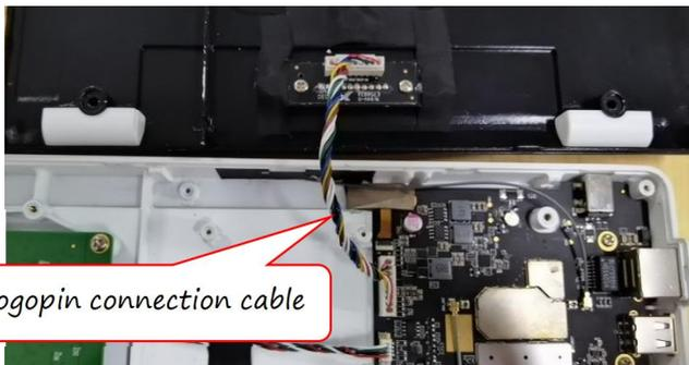
2. Align the rear housing with the front housing and press gently to bring the front and rear housing together.
