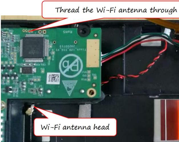
2. Snap the main control board into the corresponding position on the front housing, and fix it with 3 M1.4 \* 5 pan head non-tapping screws without any adverse phenomena such as slipping or loosening.
