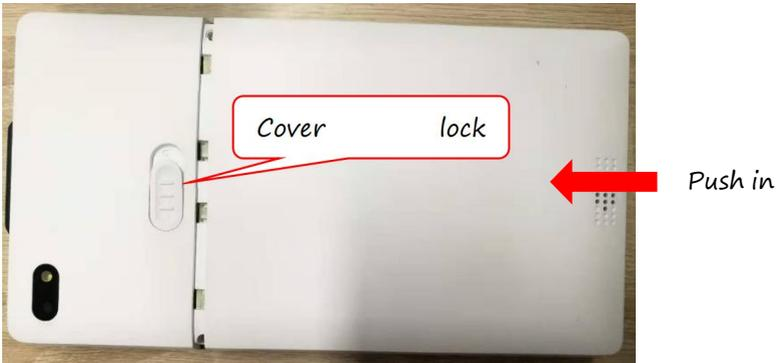
2. Flick the cover lock switch up to lock the battery cover.
