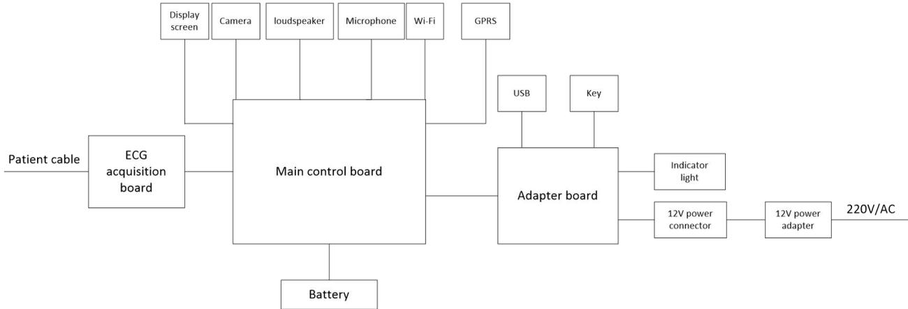
Structure block diagram of 7" model device
