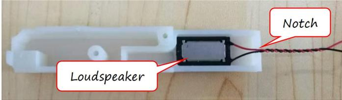
3. Install the lower cover of the loudspeaker support to the upper cover of the loudspeaker support.
