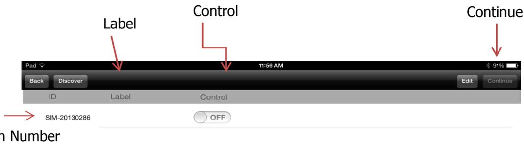
12. If you want to name your patient simulator tap the area under the "Label" column. A text box will display, that when tapped will bring up a keyboard to enter a name for the patient simulator. After you type the name, tap the 'Done' button on the keyboard to save it.
