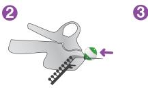
Insert fasteners into the Fixxon gun, using the bottom slot. Push until they 'click' into place.
