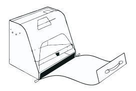
2. Unzip the front and fold under the base of the UV GlowBag.
