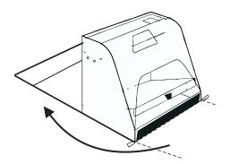
3. Switch on the Glowbar UV lamp in the top of the UV GlowBag and it is ready to use.
