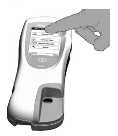
You can open any displayed function by touching (or tapping) the button for it with your finger (or a special pen for this purpose). "Tap" means: Touch the button, then remove your finger from the touchscreen. The next screen appears once you remove your finger.
