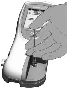
**5** Apply the entire sample to the sample application area of the test strip.
