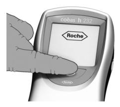
Power the meter on by pressing the button for approximately 1 second.
