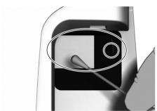
1 Clean the easily accessible and visible pipetting field area of the test strip guide with a moistened cotton swab/bud or tissue. Then dry the test strip guide with a fresh tissue.
