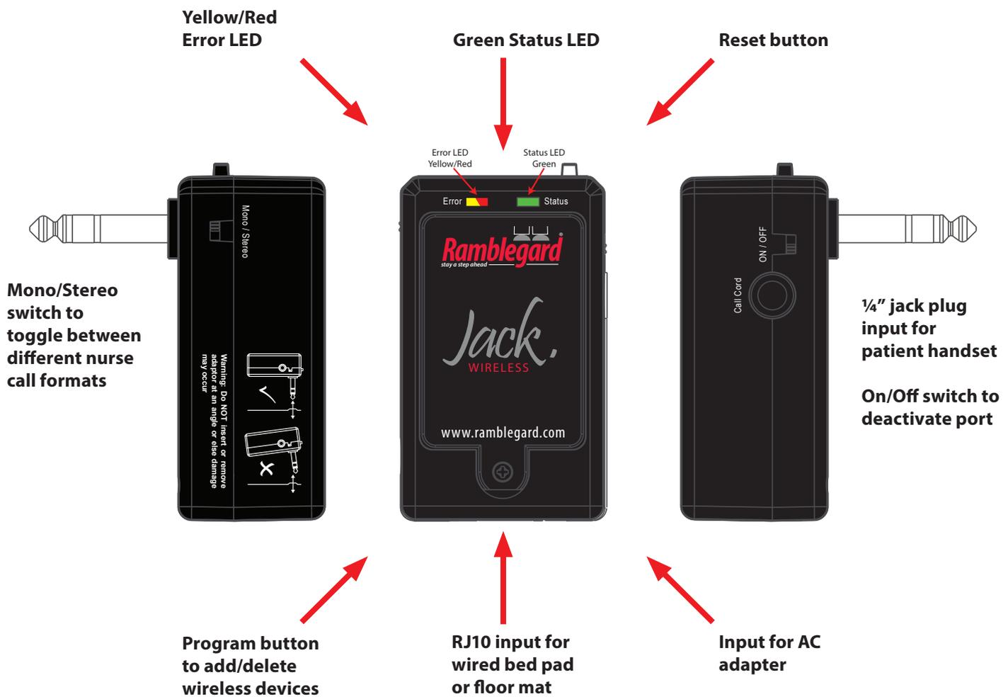
The Ramblegard Wireless Jack™ (RG5) will increase the functionality of existing communication systems by allowing wireless devices to output alarms signals into a nurse call panel. This will allow easy integration of Wireless bed and floor mat sensors for fall management, and Wireless call buttons.
