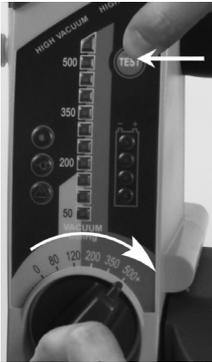
**Note:** Do not release the TEST-Button until min. 2 seconds after the Operating Knob has been set to 500+ mmHg. The test will start immediately
